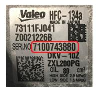
In this example (710043880), the "7" indicates the production year as 2017 (an "8" would be 2018, etc.). The next 2 digits, "10" indicates October as the production month (a "09" would be September, etc.). NOTE: Any compressor with a production date of 810 or HIGHER (October 2018 or newer) had the new valve component installed at manufacture and does NOT require replacement.
