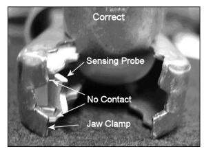
There must be no contact between the inside connection and outside jaw of clamp -arrows-.
