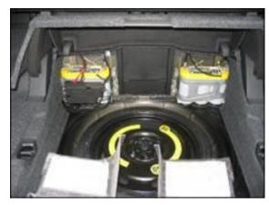
(3.2L) Test/charge AGM battery located in trunk - one 6V battery located on each side of ski chute, as shown.
