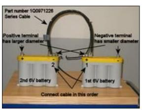
• Connect cable (Part No: 1Q0971226) to inner battery terminals.
