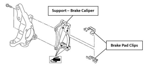
• Before installing new brake pads, remove the pad clips and **thoroughly** clean the caliper support of any dirt, rust or corrosion, paying close attention to the areas where the clips are attached / seated.
