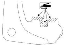
• Apply a thin coating of brake grease to the ends of the new brake pads where they contact the pad clips.
