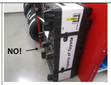
Do not place HV Battery this way as electrolyte leak may occur
