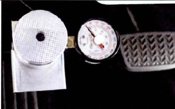
Brake pedal force gauge: SST 09709-00002
